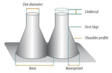
The three-dimensional screen dot shape is defined in the PremiumProfiler. Various parameters determining the shape of the screen dot can be defined here for a number of tonal value areas. The defined parameters are saved in profiles in the PremiumProfiler and are available for further use.
